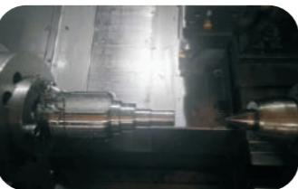
WS8135 with GM chip-breaker, provide strong versatility for ultra-high speed finish turning of workpiece with both continuous and interrupted machining requirements.
