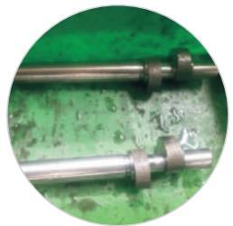
T type chip breaker, smooth and light cutting, effectively reduced the vibration.special designed grade WS8133 provide good vibration resistance, excellent wear resistance and stability.
