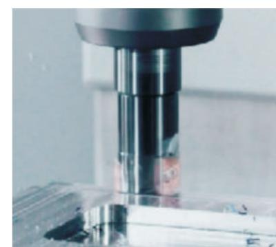
Excellent sidewall surface finish, runout <0.005mm
