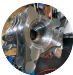
HS8125 with GM chip breaker, provide strong versatility for heavy interrupted rough turning from fixed speed to variable speed.
