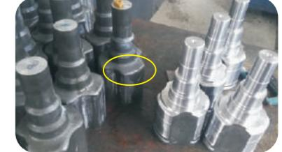
HS8125 with MT chip breaker, provide strong versatility for medium speed rough turning of interrupted workpiece.
