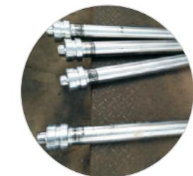
Suitable for low speed rough turning with large cutting depth and high feed. typically used to solve the low toughness problem of long slender rod machining, or low speed hard material machining, or soft material with large cutting depth.
