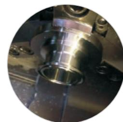
BF chip breaker, with sharp edge, landless design, big and wide rake angle, provide small chip deformation and small cutting vibration, suitable for fine machining with high surface quality requirement only.
