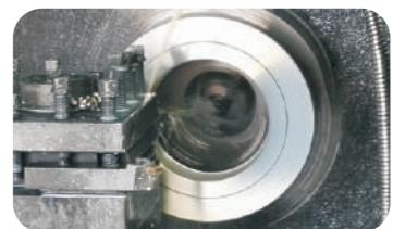
BM chip breaker, belongs to general-purpose chip-breaker, provide very good performance under various environment, except for rough turning on oxide coating which has no obvious advantage.
