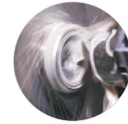
T chip breaker provide excellent chip evacuation control for stainless steel machining.
