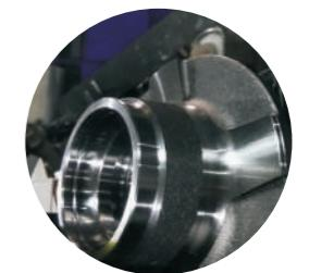
HS8115 with MT chip breaker, has good performance for high speed continuous turning of inner hole with poor cooling effect.
